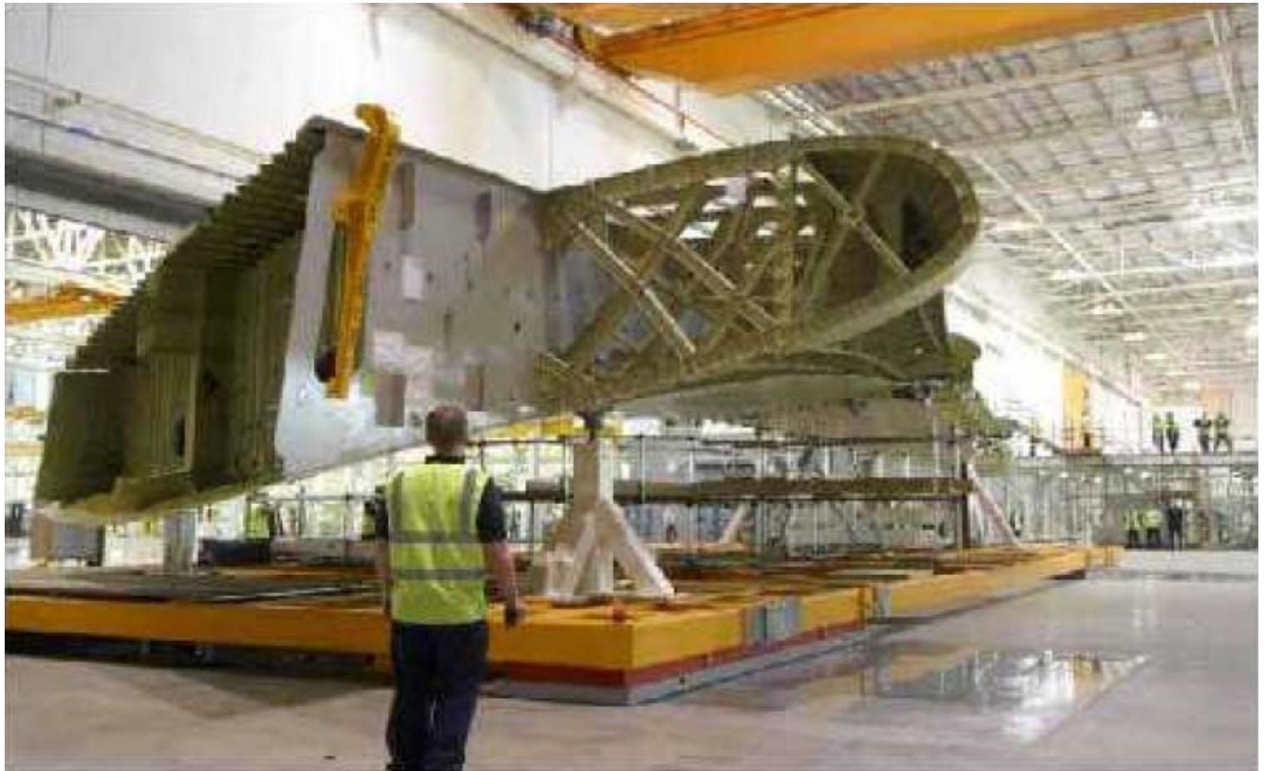
Based on computational results for maximum stiffness and quite a bit of engineering interpretation a new type of structure was devised for the ribs which gave a weight benefit against traditional and competitive honeycomb/ composite designs (up to 40% !)
