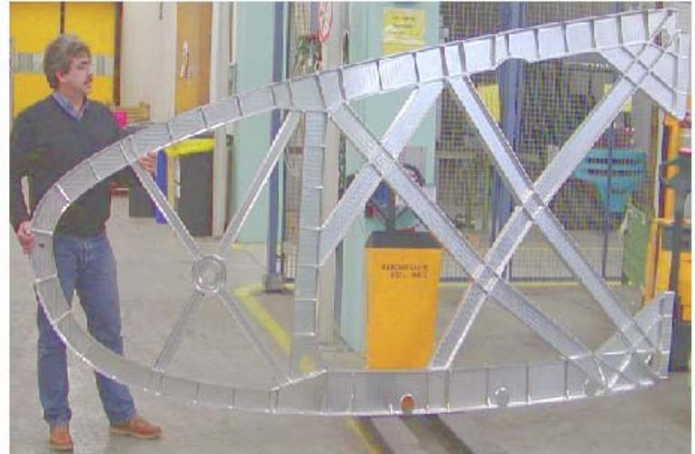
Wing element for Aerobus A380
