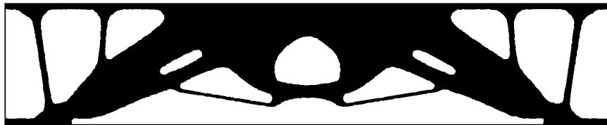
FIGURE 1 – An optimized shape for a 2-d bridge featuring 10 load constraints (from [1]).
