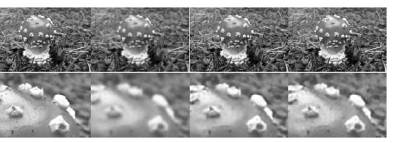
Figure 3.: Deblurring results with blur factor  $\tau = 1.5$  and Gaussian noise with  $\sigma = 0.01$  using FBS-PnP with a cPNN based denoiser and  $L_2$ -TV.
